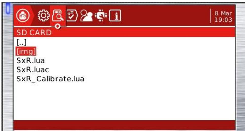
Select **SxR\_Calibrate** and execute it. The yellow light should flash whilst each part of the calibrating process is taking place.
