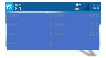
All of the values are shown in gray, even though the color is set to black. That's because the airplane is not on, and no data is being sent. When the airplane is functioning, the screen looks better.
