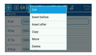
I'm going to use Switch SD for changing between high and low rates. Edit the settings for Ail so that the settings are effective for Switch SD in the up position. Also add 10% expo (as suggested by the plane's manual).
