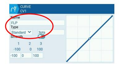
The manual for this plane tells us that the three positions should be -100%, 0%, and +100%. That's how the curve is set by default, so we'll leave it set that way and stop here. If your plane has different settings, or you want to adjust them later, you'd change the values in this curve.
