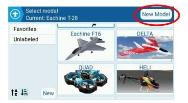
On the Select Model screen, I'm going to select "New Model" in the upper right corner. That will present a screen that gives four choices for how to create that new model.
