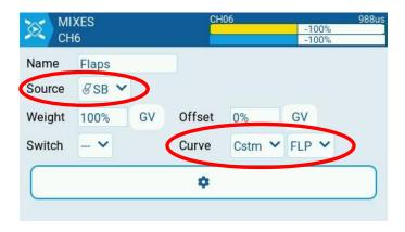
To set the movement speed, select the Gear icon to open more settings. Change both "Slow Up" and "Slow Down" to a speed that you'd prefer. I'm going to use 2.0 seconds, as that's a common recommendation on the Horizon BNF's.
