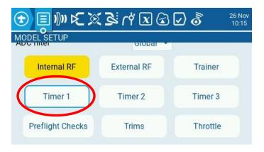
First, assign the timer a name. "Timer 1" is fine, which is the default name in Spektrum radios and the generic name for the first timer in EdgeTX.
