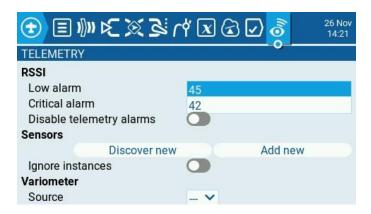
Select "Discover New" to have EdgeTX add new sensors (data elements) automatically by listening to what's being sent from the receiver.
