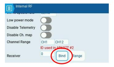
After a few moments, you'll find out if the bind was successful based on whether the receiver initializes and gives you control. Receivers with SAFE will usually take a bit of time to get ready, and they'll wiggle the control surfaces in the process.
