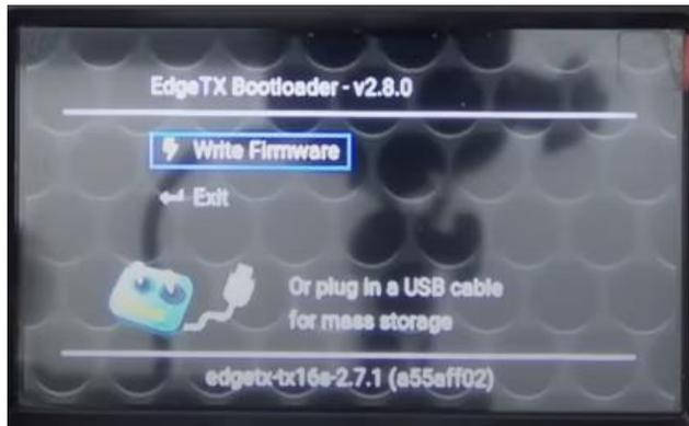
At this point, connect the USB cable, and then the SD card will be accessible from the computer.
